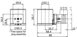
Coil with Deutsch DT04-2P plug connection
