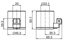
Coil with AMPSEAL 16 axial plug connection
